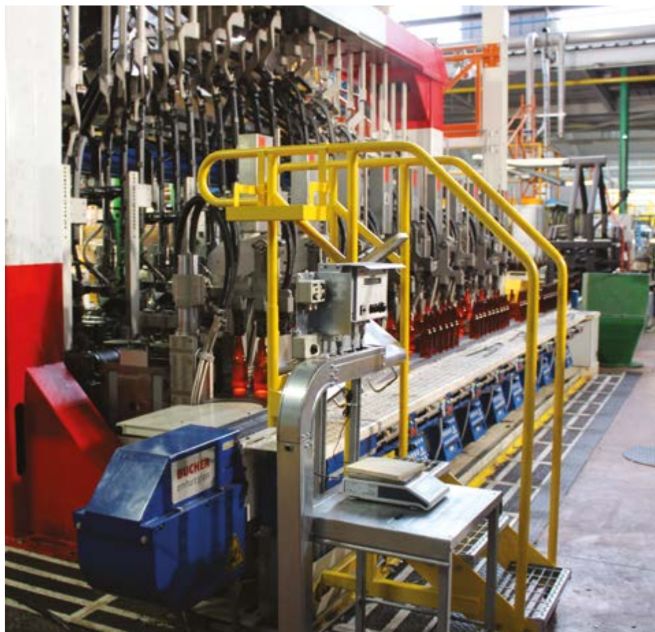
Safety ladder integrated into FlexConveyor.
